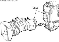
3 Lower the lens clamping lever and clamp the lens.
